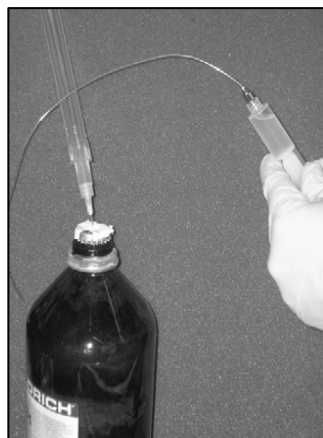
Fig. 4 Needle tip is brought into headspace of bottle and an inert gas layer is drawn into syringe needle-up to prevent spilling
