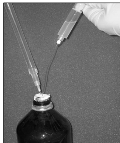
Fig. 1. Drawing reagent into syringe from reagent container, with inert gas line inserted.
